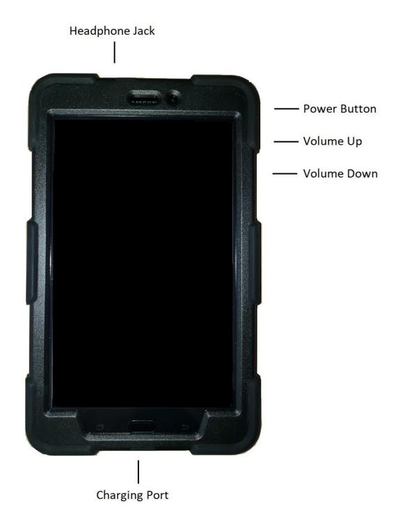
The headphone jack and charging port have small flaps to prevent dust and water damage. Open these flaps to use these ports.
